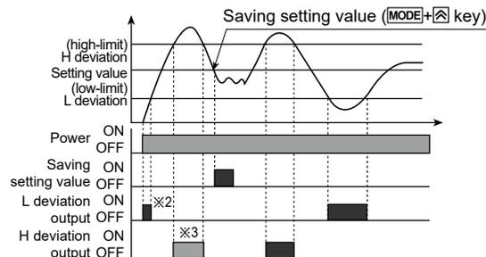
※2: When selecting initial comparative output limit function, it does not transmit outputs.
