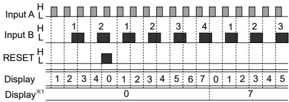
※1: When the display cycle [ $d_i$  5P.t] setting is OFF, it will maintain the quantity of input A until the value of input B reaches the setting value B[ $\alpha$  0.t.n.b].
