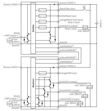
01) This wiring is used to activated the lamp output and displays the status to the external indicator based on selected output mode. 02) RS485(A) and RS485(B) are for the synchronous line.
