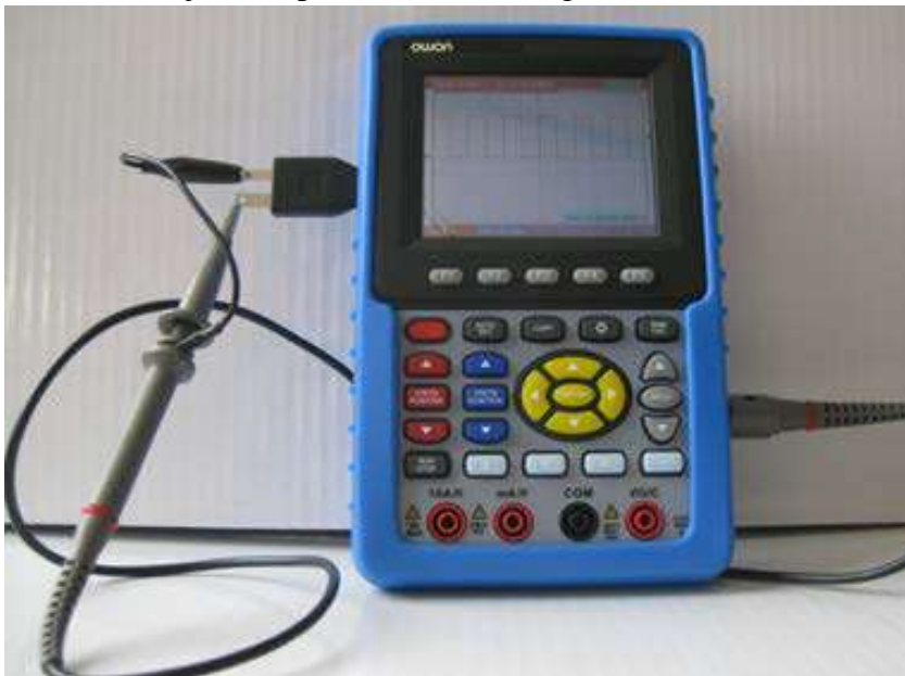
Fig.3. The connection of Square-wave test signal
